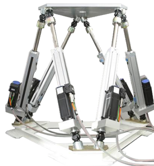
(b) Example of a parallel robot
