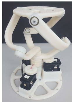
(b) Example of a parallel robot
